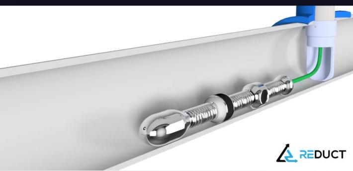
The LGM-2 a unique mapping designed to map buried live gas pipes with an ID range of 50mm up to 100mm (2" to 4"). From a single hot tap entry point it can map a gas pipe up to 300 meters/1000' length in each direction, thus capturing data and the geographical location of 600 meters/2000' of live gas pipe.
